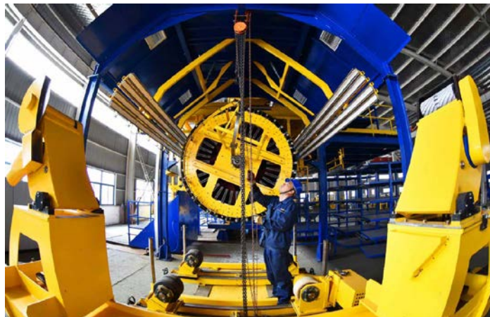
An employee installs an intelligent pipe winding machine at an industrial park in Lianyungang, Jiangsu Province. Photo: Geng Yuhe/CHINA DAILY
